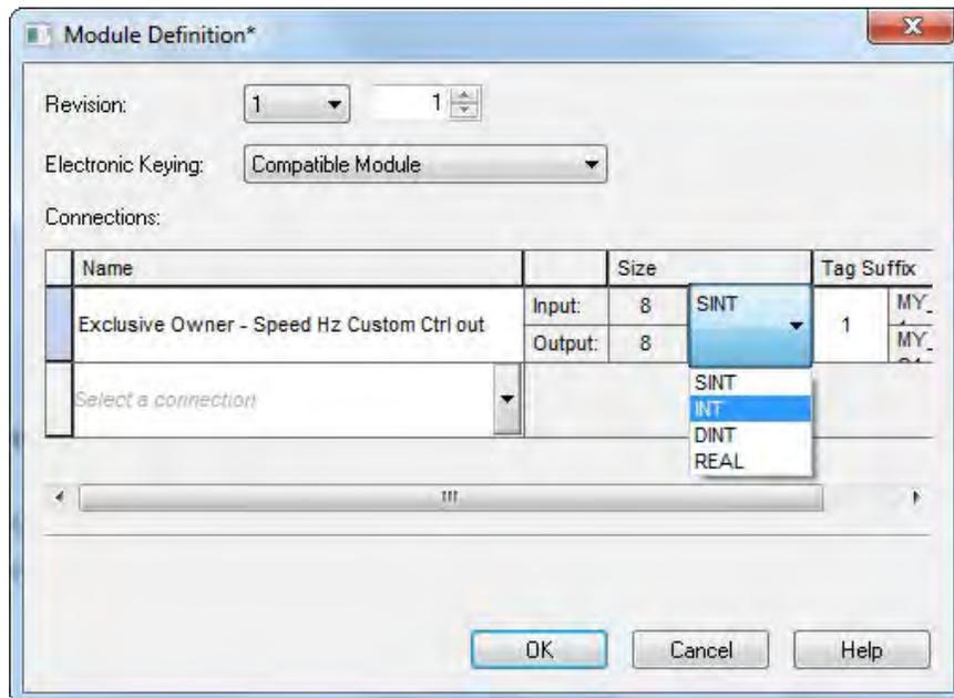
A tag suffix is used to formulate module-defined tag names. Leave this value set to the default value of “1” and click “OK”.
