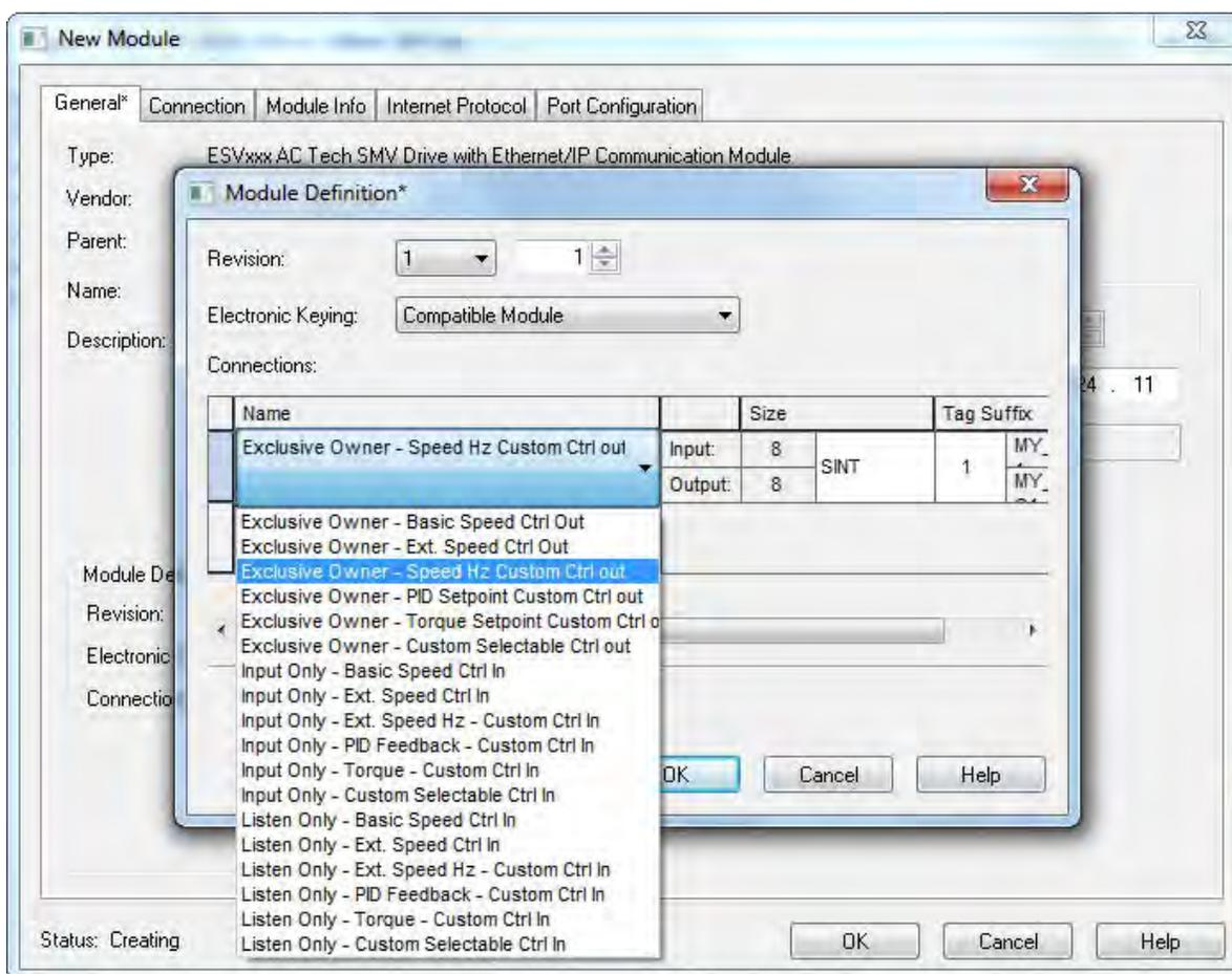
Next you need to select the data format of the assemblies you are using. Select the “INT” format as it is the easiest to work with in the Rockwell PLC for use with the SMV.
