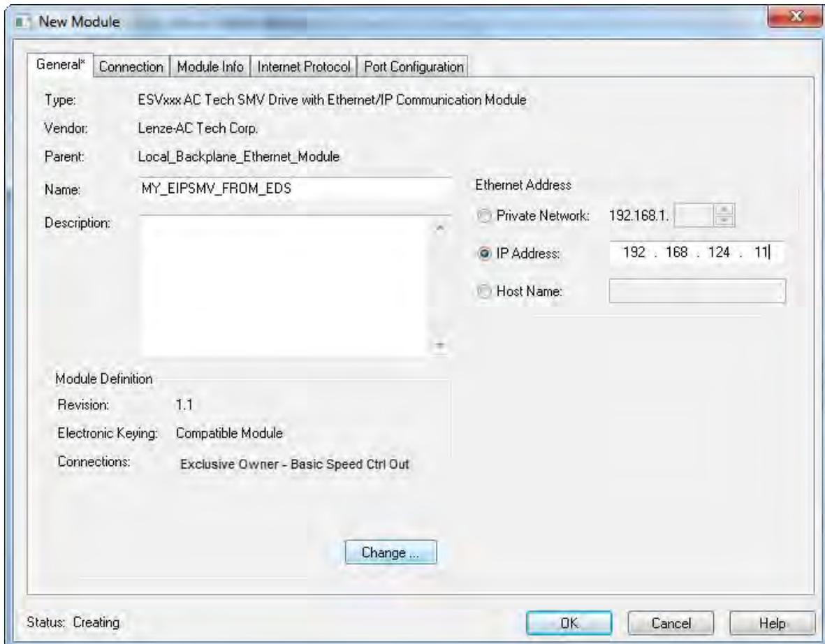
In this example (as with most applications) the PLC will be both controlling and also receiving status from the drive. We will allow access to both speed and the on board drive I/O. Set the "Name" to "Exclusive Owner – Speed Hz Custom Ctrl out". This uses assemblies 101 for status and 100 for commands to the drive.
