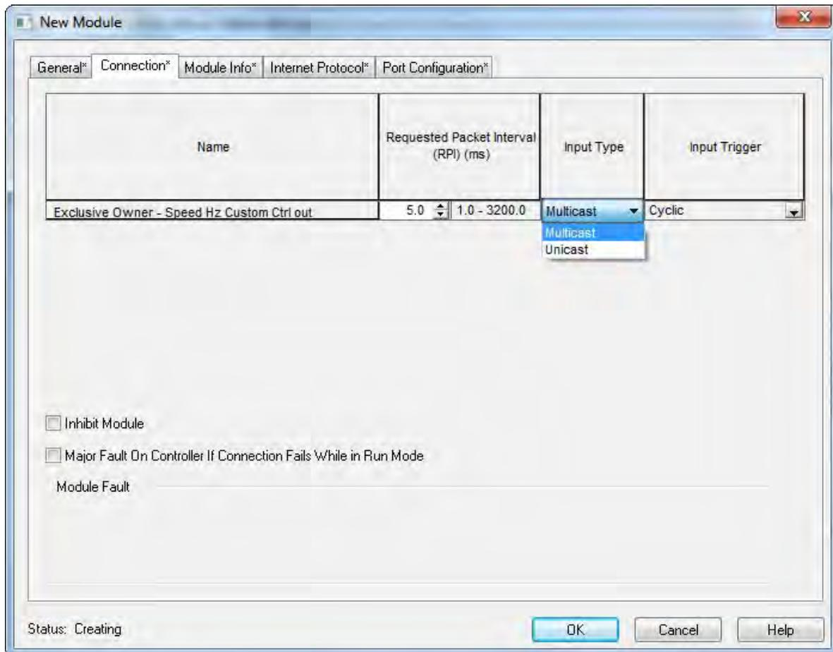
If you want the PLC to Fault if it loses communication to the SMV drive, select “Major Fault On Controller If Connection Fails While in Run Mode”.
