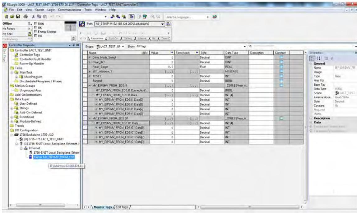
Click the “+” next to the assembly tag name to expand the menu to see the full data within each assembly. The user may then create alias tags to reference individual bits in the assembly as they would for any other alias tag in RSLogix™ 5000.
